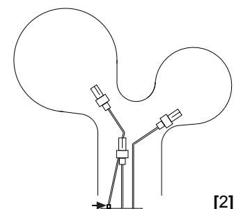
The arm is attached to the metal base with a hinged joint that is locked to position with a pin. Pull out the pin. [2]
