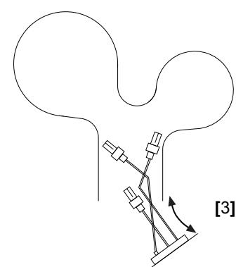
Once the metal structure is out of the Double Bubble, you can replace the bulbs.
