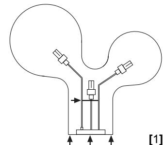
Carefully pull the metal structure out of the Double Bubble until you can reach into the lamp.
